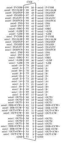
Axis0 - Axis3 of this manual corresponds to Axis No.1 - Axis No.4 in API-SMC(WDM).
