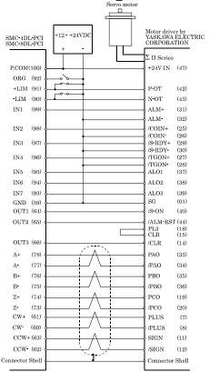
\* Please connect the Shield Line of cable with the Connector Shell.
